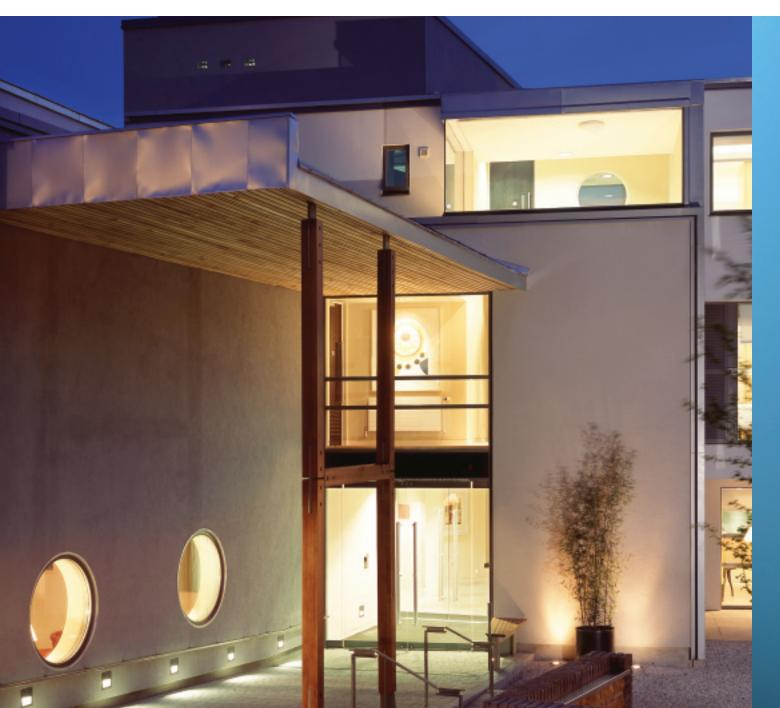
With carefully chosen light fittings and lamp sources a multi-channel lighting scheme can enable the mood and function of a space to be changed, highlighting features and creating pockets and pools of light. Scene control dimming allows these new moods to be re-called at the touch of a button and with the possibility of multi-way control, hand-held remotes and integration with security and audio visual systems a home moves to a new level of sophistication.
